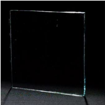
The haze reading for Clarvista glass in a clear glass substrate after pH/jungle box testing with the bath/shower stain remover was less than 1 percent.
