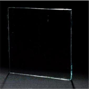
After pH/jungle box testing with baking soda, Clarvista glass in a clear glass substrate had a haze reading of less than 1 percent.
