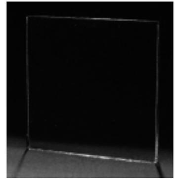
*After pH/jungle box testing with baking soda, Clarvista glass in a clear glass substrate had a haze reading of less than 1 percent.*
