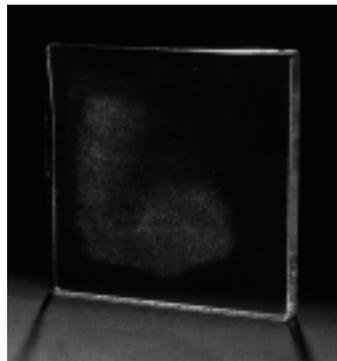
*pH/jungle box testing with the bath/shower stain remover resulted in a haze reading of 4 percent for the leading competitive coated clear glass.*
