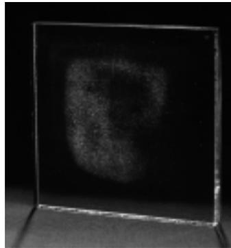
*The leading competitive coated clear glass sample had a haze reading of 3 percent after pH/jungle box testing with the ammonia-based glass cleaner.*
