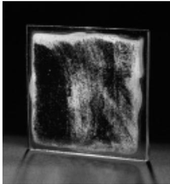
*pH/jungle box testing with baking soda generated a haze reading of 61 percent for uncoated clear glass.*
