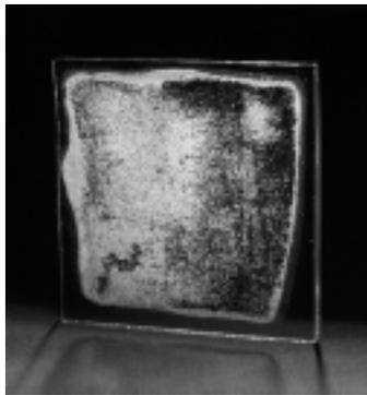
*pH/jungle box testing with the ammonia-based glass cleaner created a haze reading of 87 percent on uncoated clear glass.*
