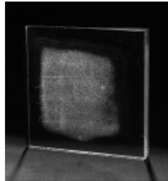
*On the leading competitive coated clear glass, pH/jungle box testing with baking soda produced a haze reading of 22 percent.*
