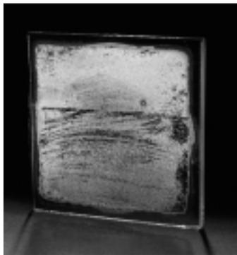
*pH/jungle box testing with the bath/shower stain remover produced a haze reading of 70 percent for uncoated clear glass.*
